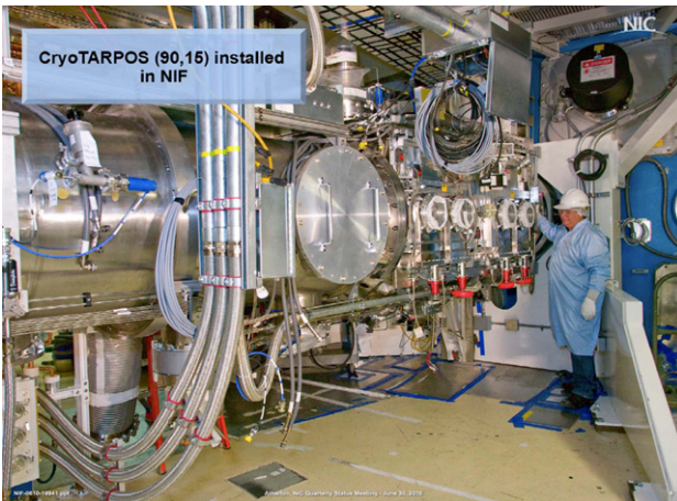
Figure 6. Cryo-tarpos enables the formation of cryogenic layers just outside the NIF target chamber.
